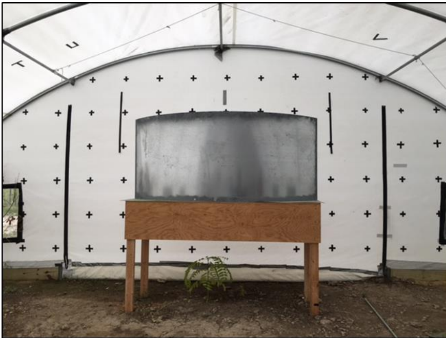
Figure 8: Image of the replica portion of a wind turbine tower used in bat foraging behavioral trials in the flight facility.
