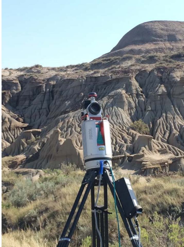
Figure 14: Photo of Riegl VZ-400 LiDAR scanner with Nikon D700 SLR camera mounted above.
