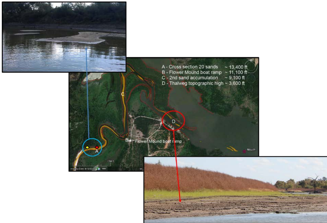
Fig. 17: Aerial image of the Denton Creek Delta with channel sand locations overlain as orange polygons. Tomanka found that sand in Denton Creek was trapped upstream as bars and the river mouth was predominantly soft clay in comparison (Tomanka, 2013).
