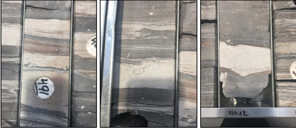
Fig. 41: Noblige-2 core of the Mungaroo Formation, Western Australia. These thin sands may be blowout wings and have the potential to improve reservoir connectivity.
