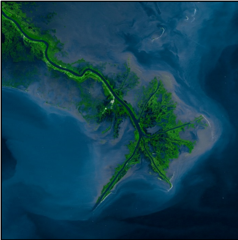
Fig. 7: The modern birdsfoot lobe of the Mississippi Delta is a common example of a fluvial-dominated delta, where the elongated morphology is influenced by the discharge from the river system (image courtesy NASA Visible Earth)
