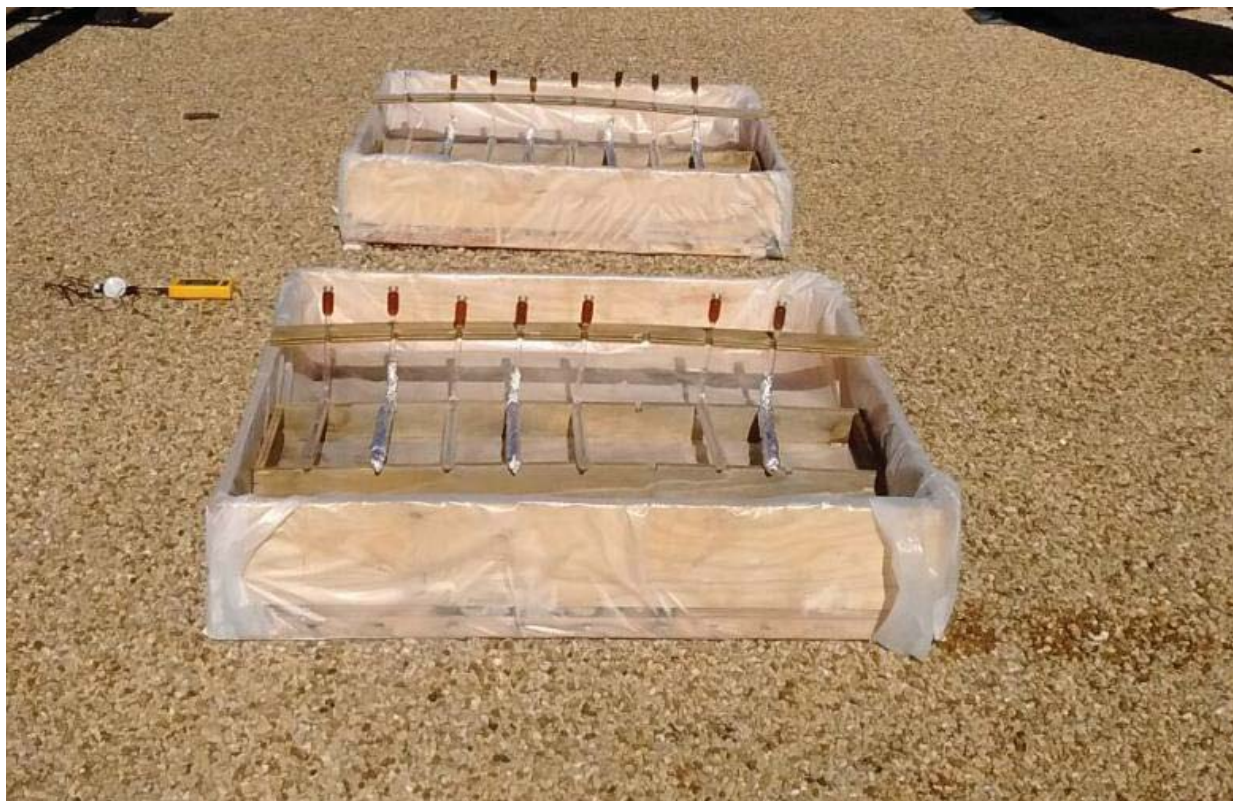
Figure 11. Quartz tubes containing Py -DOM/DOM extracts of Eastern Cedar and extracts exposed to solar radiation. Solar irradiance meter (pictured in yellow) recorded at 5 minute intervals.
