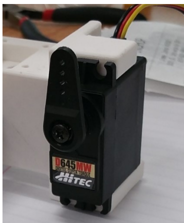
Figure 16 – Hitec D645MW Servo, placed in arm mount
