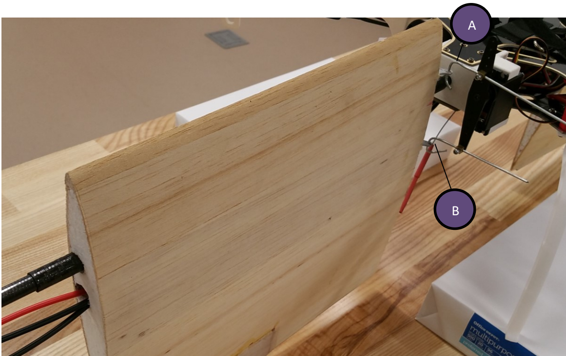
Figure 18 – Operational Wing Rotation System
