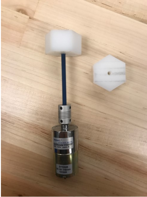
Figure 15: Plastic hexagonal shafts are tapped and screwed onto the threaded rods.
