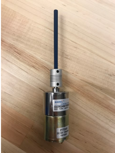
Figure 13: A coupler connects the head of the DC motor to the threaded rod.
