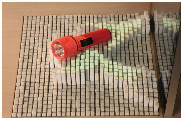
Figure 2: InFORM Surface projecting hands holding a flashlight. Image credit: InFORM. http://tangible.media.mit.edu/project/inform/ .
