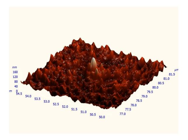
Figure S2: Dye doped PVA layer thickness on the glass coverslip using AFM.
