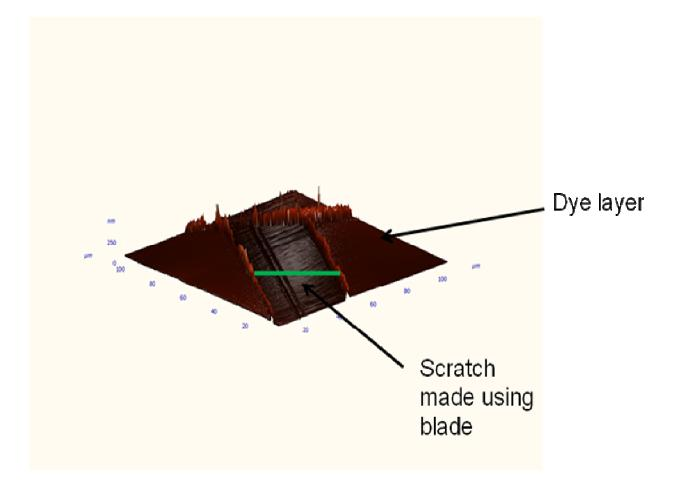
Figure S3: Height profile across the scratch made on the dye layer from Figure S2.
