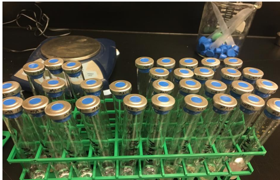
Figure 3. Sealed and crimped reactors prior to autoclaving, inoculation, and pressurizing with H 2 /CO 2 or N 2 /CO 2 gas.
