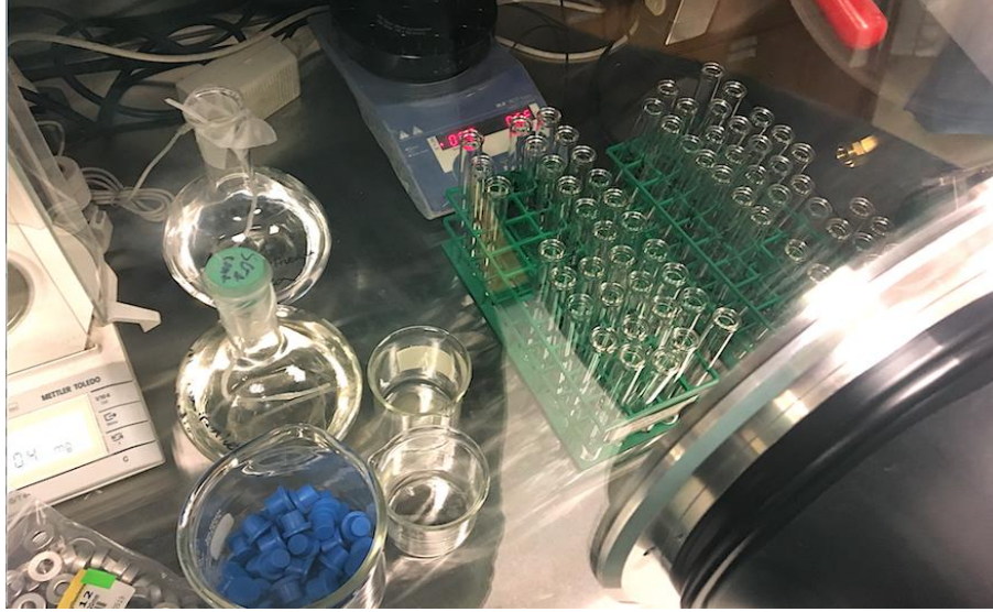
Figure 2. Experimental Setup in Anaerobic Chamber where media was transferred to “Balch” tubes with varying treatments followed by crimping and sealing.
