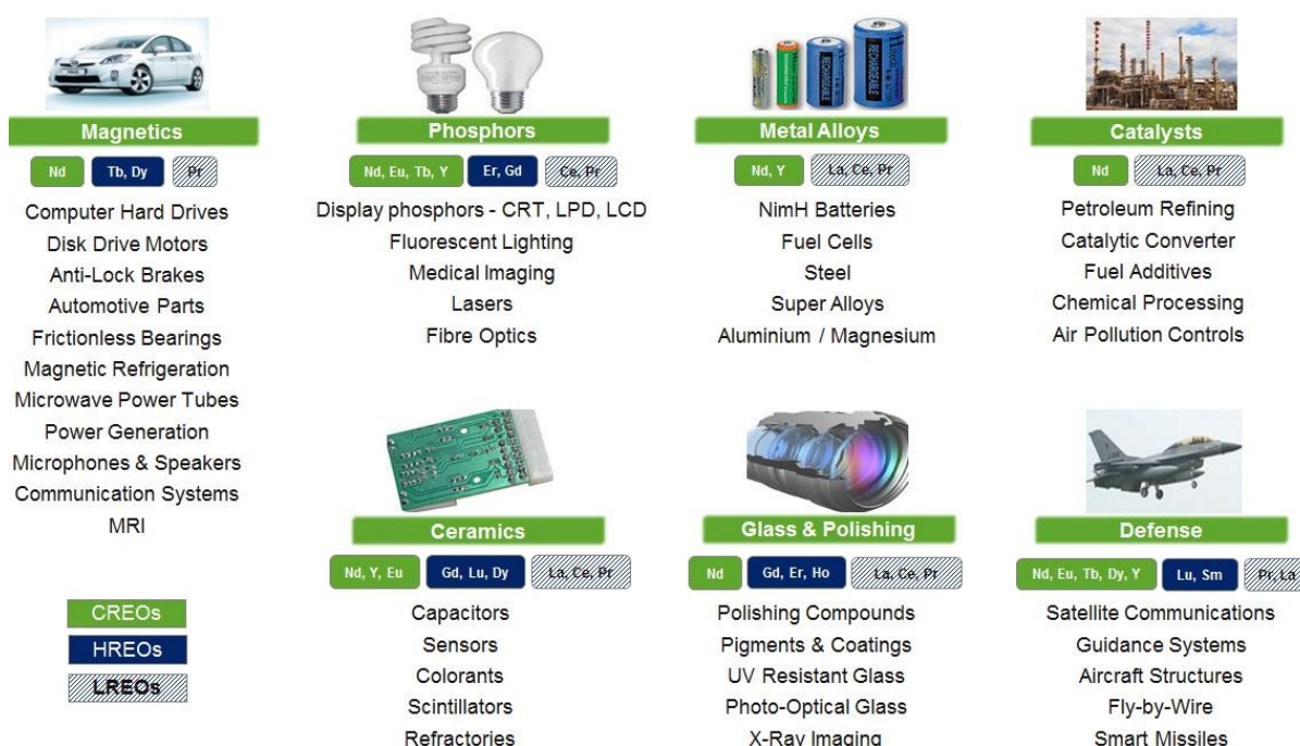
Figure 8: An Array of the Many Uses of Rare Earth Elements Divided into Categories
