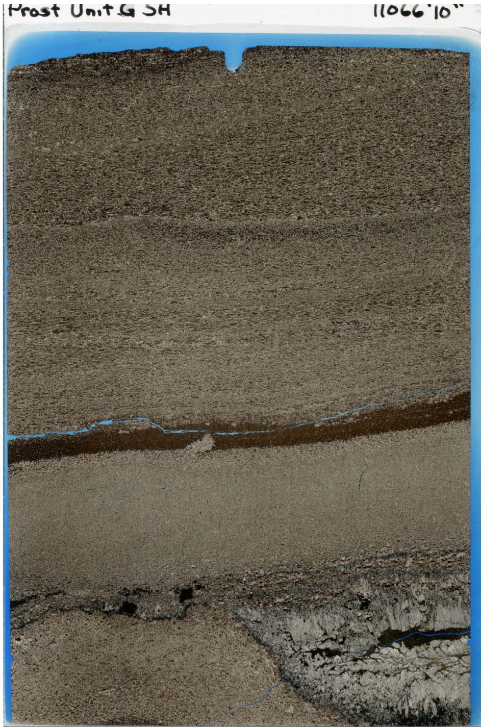
11066'10" - fibrous calcite encasing ash bed; recrystallized laminated limestone
