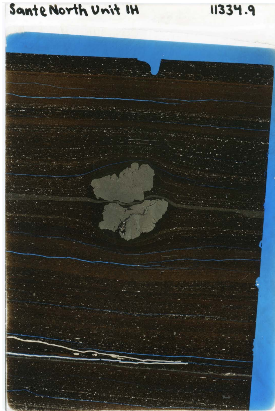
11334'9" - alternating massive argillaceous mudstone interbedded with indistinctly laminated mudstone with sizeable pyrite nodules with a thin ash bed and inoceramids. Taken under reflected light.
