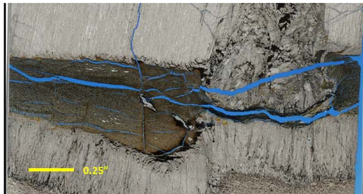
FIGURE 27. MICROFACIES e - SCANNED IMAGE OF THIN SECTION WITH TRANSMITTED LIGHT DISPLAYING CALCISPHERE PACKSTONE (0.25 IN = 0.64 CM).
