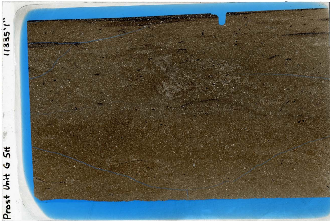
11335'1" - massive Limestone, mottled to massively bioturbated with calcispheres, benthic/agglutinated foraminifera, ostracods
