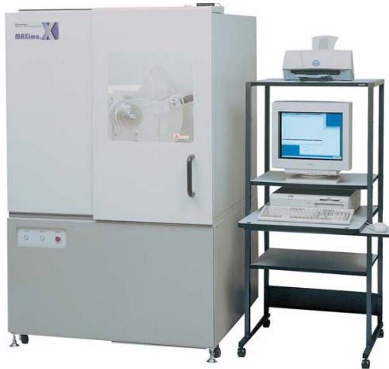
FIGURE 14. THE MAXIMA X XRD X-RAY DIFFRACTOMETER HAS A CONTAINED TESTING AND ASSOCIATED COMPUTER APPLICATION FOR ANALYSIS (SHIMADZU CENTER, 2014).
