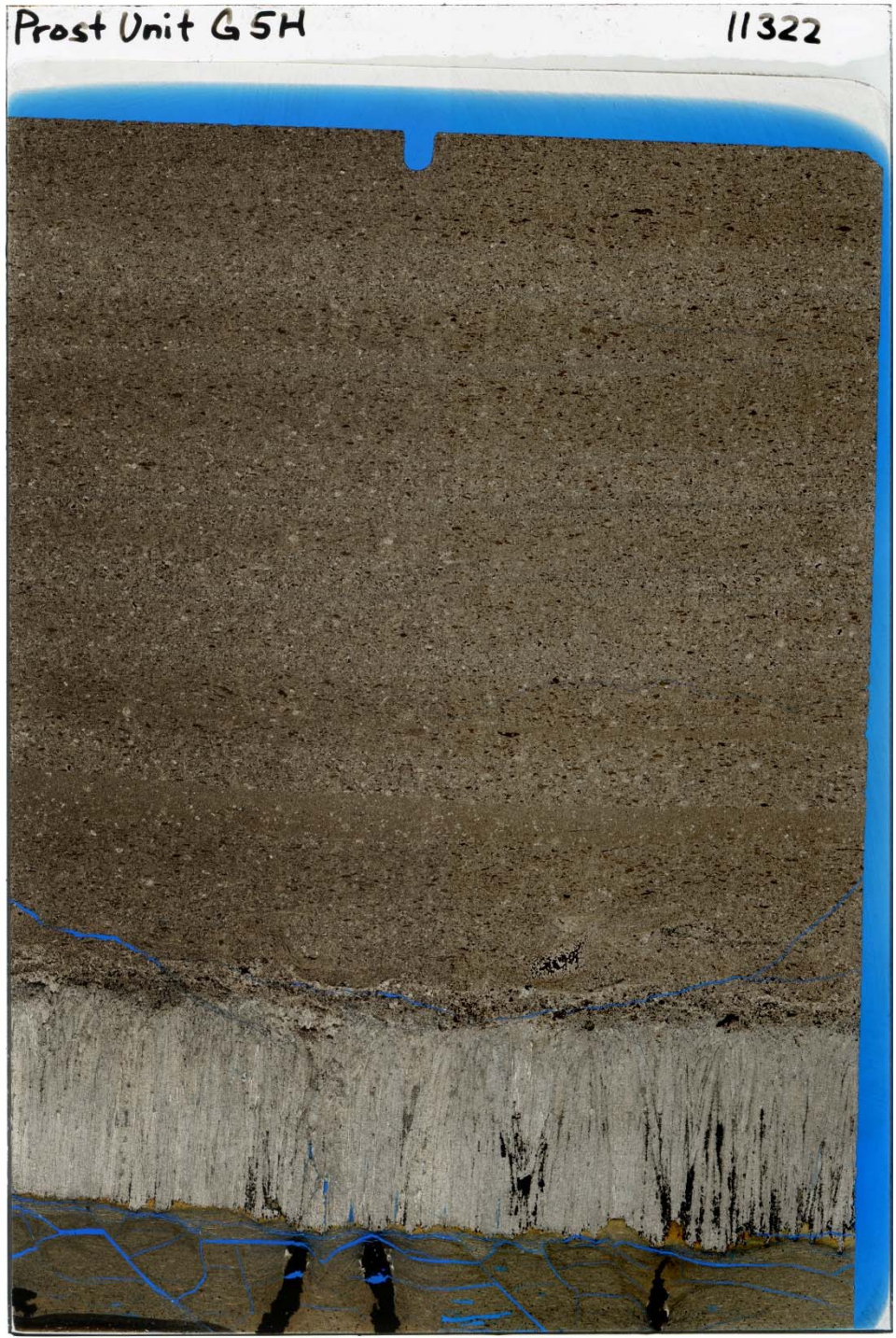
11322'0"- recrystallized laminated limestone; large (1cm) fibrous calcite; ash bed
