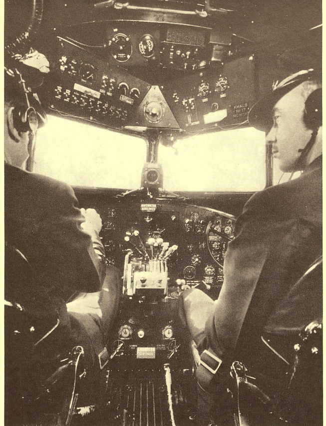
The instrument panel of a DC-3—The two Argon lights mounted on the front of the control pedestal are barely discernible in the picture
