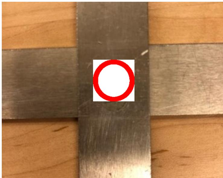
*Figure 8: Clutch point in open position. The red circle represents the location of a pin.*
