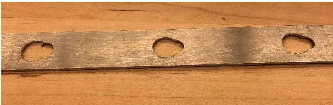
*Figure 6: Single clutch bar with holes for pins*
