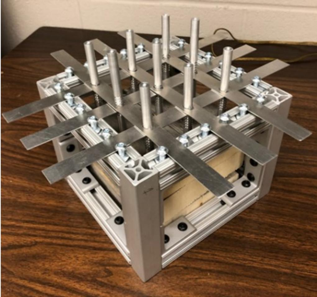
*Figure 9: Sliding bar clutch with pins mounted on T-slot frame.*
