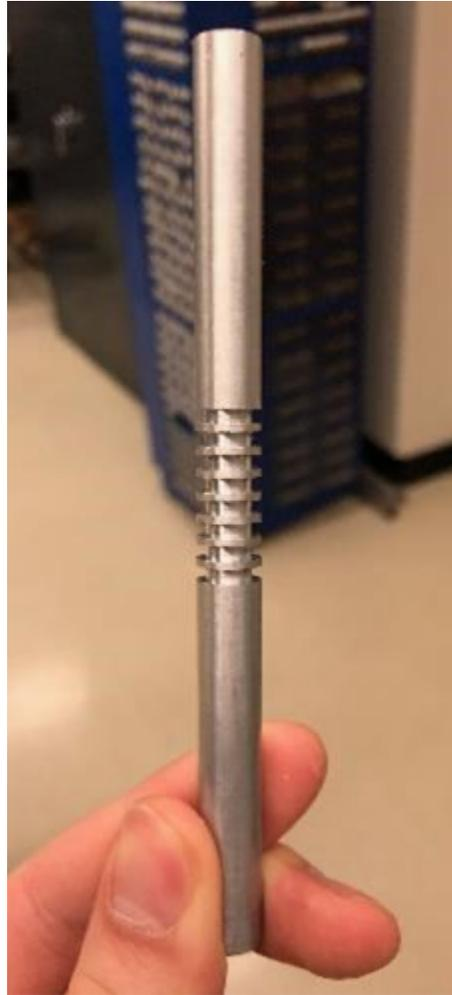
*Figure 5: Single pin element with grooves cut for clutch*
