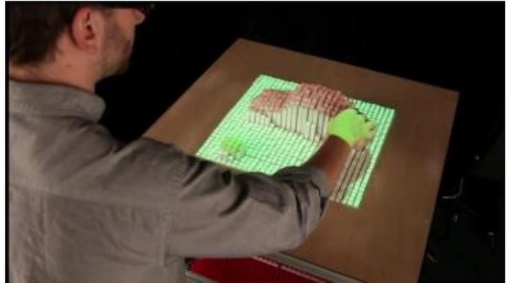
*Figure 2: inForm surface being used to alter the design of a car
