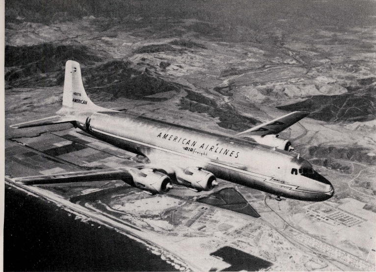
THE LATEST TO JOIN THE A. A. FLEET THIS DC-6A AIRFREIGHTER CAPABLE OF CARRYING A 28,500 POUND PAYLOAD OVER LONG DISTANCES IS NOW IN SERVICE.
