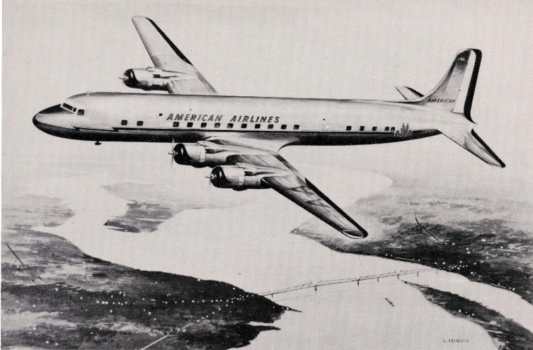
DC-7 FLAGSHIP SEATS 60 PASSENGERS AND CRUISES AT 363 MILES PER HOUR. AMERICAN WILL START DC-7 SERVICE TRANSCONTINENTALLY IN 1954.
