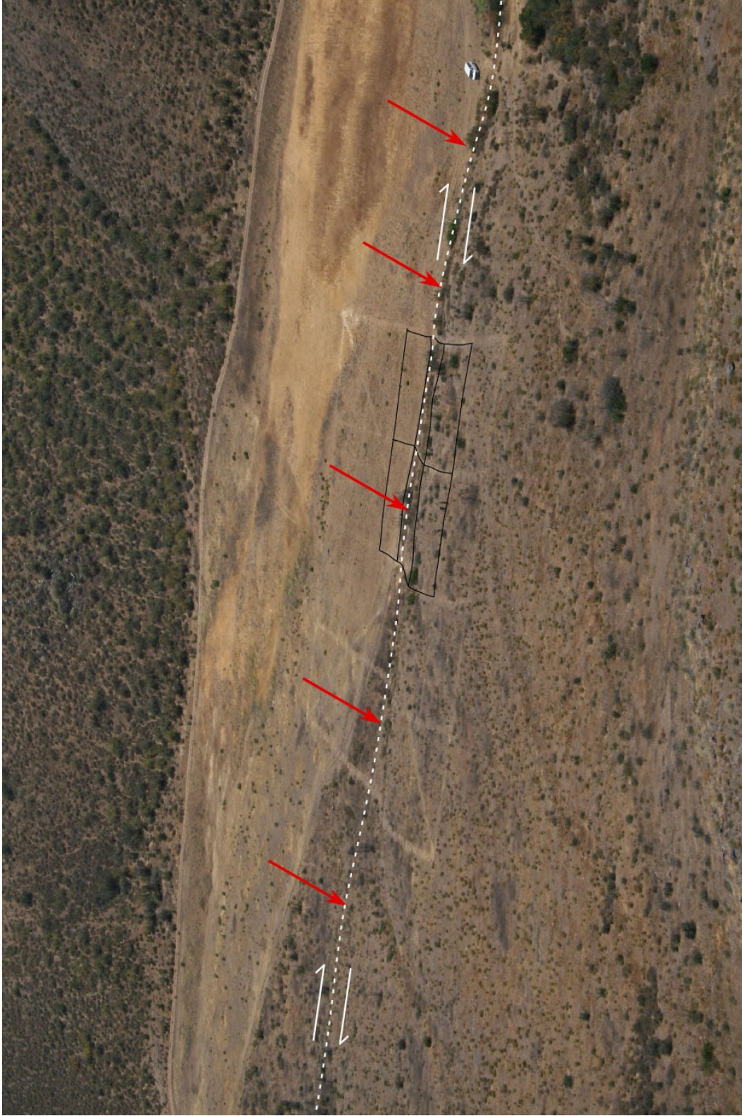
Figure 21. Location of GPR Site 2 viewed towards the south. Red arrows point to the fault scarp; white dashed line shows the fault trace; black lines show the outline of the GPR grid. The grid of Kretzer (2010) is visible in the vegetation. Van for scale on right side (west) of the picture.
