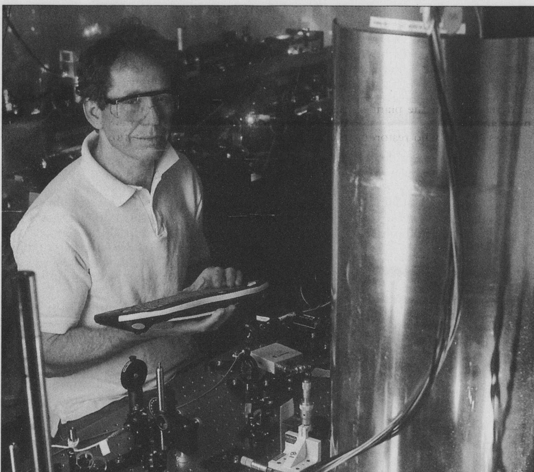
Jim Bergquist, a physicist at the National Institute of Standards and Technology in Boulder, Colo., holds a keyboard to control the world's most accurate clock. It's based on the "ticks" produced by a single atom of mercury contained at near-absolute zero temperature in the silver cylinder.
