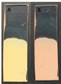
Figure 9. Photographs of the progression of a \text{Sn}_3\text{O}_4 photoanode from (A) the undyed surface to (B) the dyed sample.
