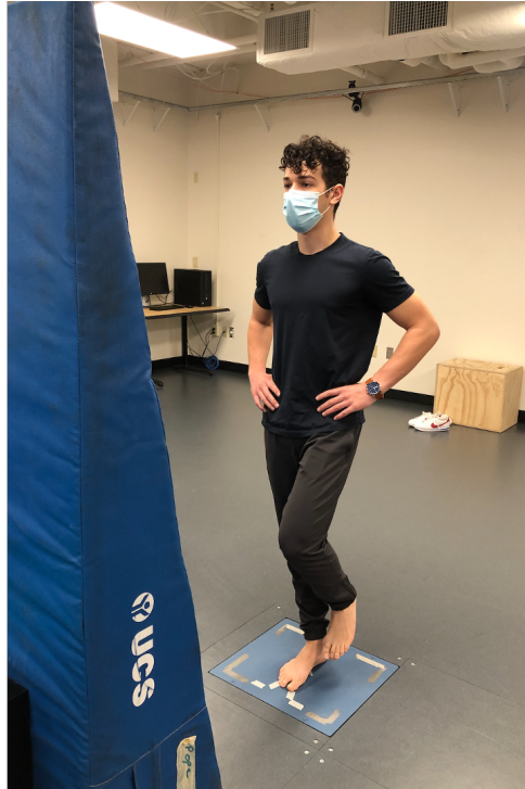
Figure 3. Participant demonstrates proper balance stance with unilateral foot on the center of the force plate, non-weight bearing leg relaxed in 90-degree position, hands resting on hips, and gaze forward at eye height.
