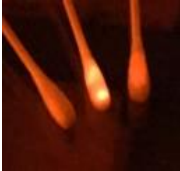
Figure 6.1. Photography of three collecting swabs. The swabs were illuminated by a 535 nm laser as seen by the 575 nm long pass filter. DNA was put in two spots on the middle swab. EtBr was then applied to the center and right swab.
