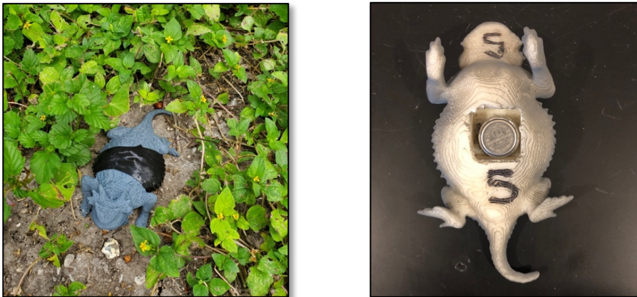
Figure 1: Horned lizard model equip with a DS1922L Thermochron™ temperature logger embedded in the belly area to approximate T_e available to lizards.
