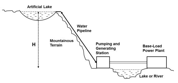
Figure 3. Schematic representation of a PHS.
