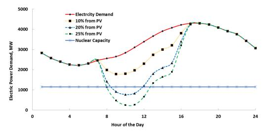
**Figure 1.** The duck curve resulting when the PV-generated electricity reached 10%, 20% and 25% of the annually generated electricity in the San Antonio, Texas region.
