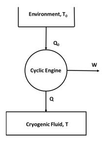
Figure 10. A cyclic heat engine operating with two heat sources: the environment and a cryogenic fluid.
