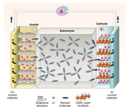
reduction reaction takes place in the cathode, where the Li<sup>+</sup> ions combine with the electrons that flow through the external circuit, a process known as intercalation.
