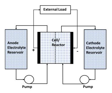
Figure 7. Schematic diagram of a flow battery.
