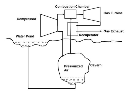
Figure 4. Schematic diagram of a CAES with a water pond to maintain constant pressure.
