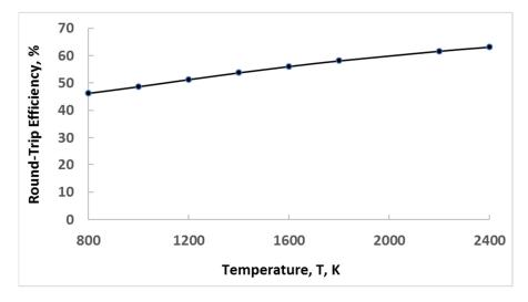
Figure 5. Round-trip efficiency of a CAES at 80 bar with variable turbine inlet temperature.
