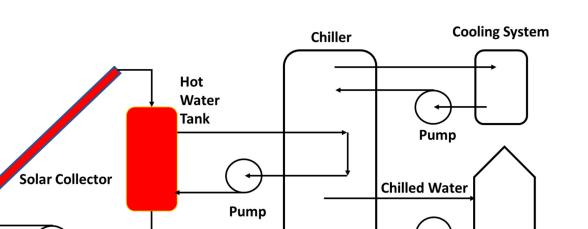
Figure 8. Schematic diagram of solar cooling with an absorption refrigeration cycle.
