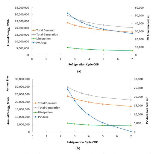
**Figure 3.** (a) Photovoltaics area needed, annual energy demand, supply, and dissipation as a function of the COP when one wind turbine is employed. (b) Photovoltaics area needed, annual energy demand, supply, and dissipation as a function of the COP when two wind turbines are employed.
