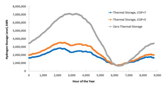
Figure 5. The level of hydrogen storage throughout the year with and without thermal energy storage.
