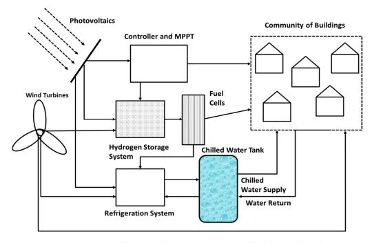
**Figure 2.** Schematic diagram of the grid-independent community of buildings with hydrogen storage and thermal energy storage.
