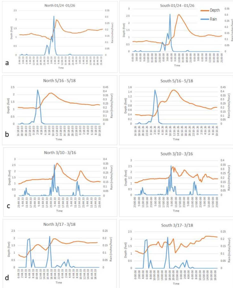
Figure 10: Examples of changes in water depth with rainfall \geq 0.80 inches. a) Single peak 0.913-inch rainfall over 9 hours, which resulted in a depth change of 1.08 feet at the north location and 2.17 feet at the south location. b) Single peak 0.976-inch rainfall over 11 hours, which resulted in a depth change of 1.05 feet at the north location and 1.15 feet at the south location. c) Multiple peak 2.29-inch rainfall over 25 hours, which resulted in a depth change of 1.68 feet at the north location and 1.37 feet at the south location. d) Multiple peak 0.88-inch rainfall over 25 hours, which resulted in a depth change of 1.27 feet at the north location and 1.20 feet at the south location.
