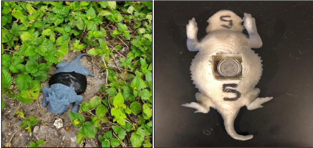
Figure 3: Left) Horned lizard model equipped with a DS1922L Thermochron™ temperature logger embedded in the belly area and secured with black self-fusing repair tape in open ground. Right) Model with temperature logger to approximate T_e available to lizards (Photos by MR Tucker).
