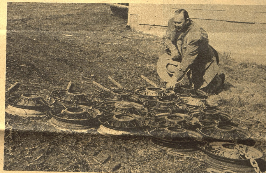
Here is Whiteman with a pasture drag he devised with old auto wheels.
