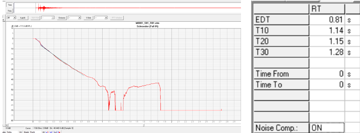
Figure 5. Example Reverberation Time Measurements from Schroeder Curves for Creekview High School Auditorium
