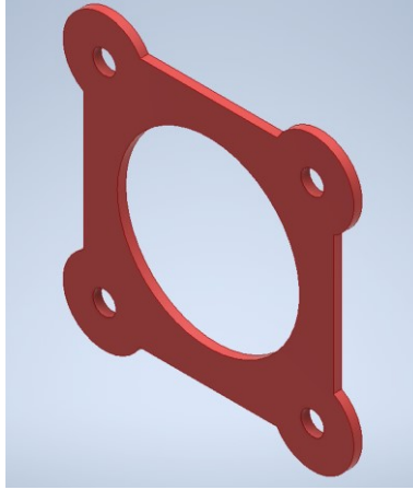
Figure 13: CAD File- Syringe Gasket Seal
