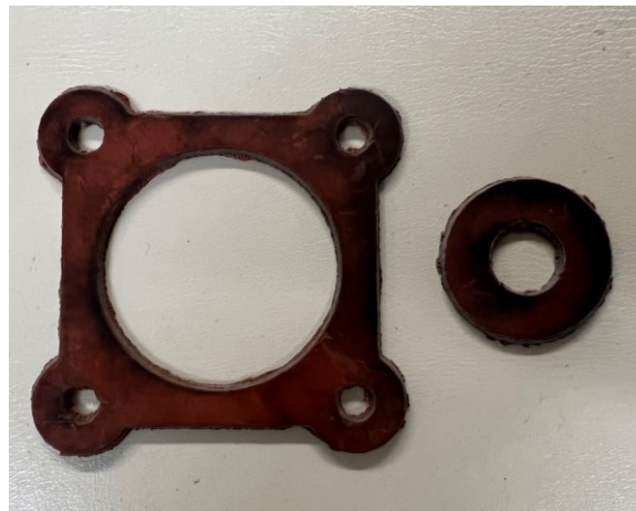
Figure 15: Actual Syringe Gasket and Compound Pressure Gauge Seal
