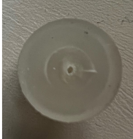
Figure 9: Laser cut TPE Cap
