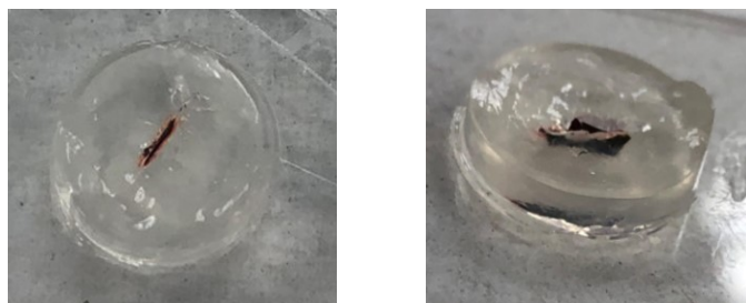
Figure 23. R6G-loaded pSi membranes physically entrapped in alginate hydrogels.
