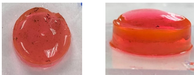
Figure 21. R6G-loaded pSi nanoparticles physically entrapped in alginate hydrogels.
