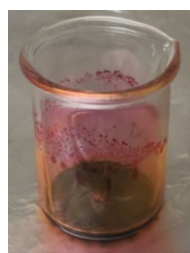
Figure 15. 20 mg pSi nanoparticles being loaded with 2 mg/mL R6G in ethanol solution.
