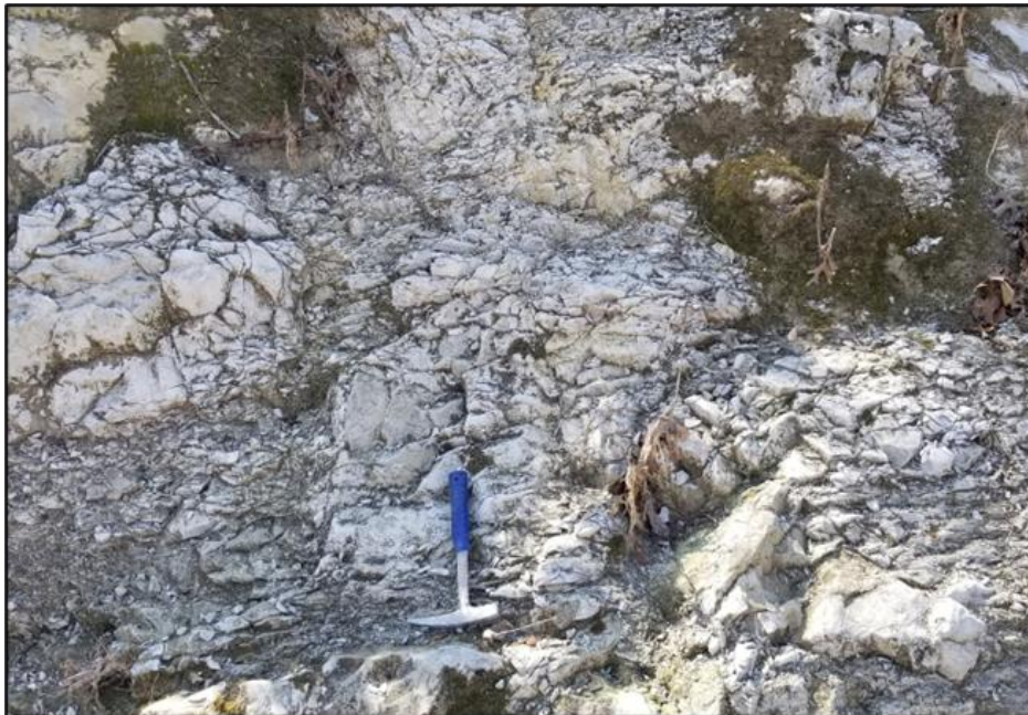
Figure 15: Brecciated fault gouge from the fault core of the normal fault observed in the Church of the Nazarene section of Ten-Mile Creek.
