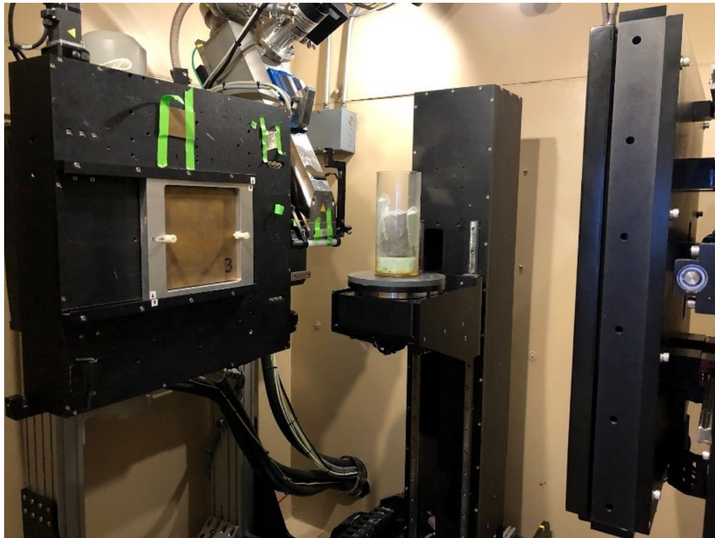
Figure 3. NSI Scanner at UTCT with the complete 800 g stone of NWA 14904 loaded into the plexiglass cylinder.
