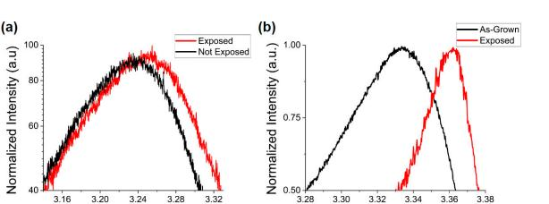
**Figure 14.** Room temperature PL spectra of the NBE region normalized to the NBE peak intensity for ZnO MPs before and after exposure to *S. aureus* in MHB: (**a**) type HP sample and (**b**) type LR sample.
