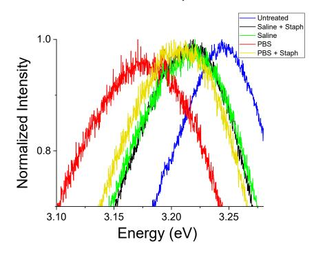
**Figure 10.** Room temperature PL spectra of the NBE region normalized to the NBE peak intensity for commercial ZnO NPs after exposure to biological environments.
