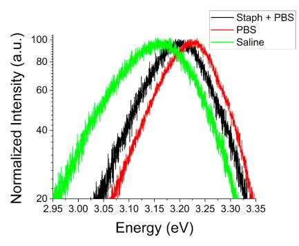
**Figure 11.** Room temperature PL spectra of the NBE region normalized to the NBE peak intensity for a type B ZnO MP sample after exposure to *S. aureus* in PBS as well as PBS and saline media in isolation.
