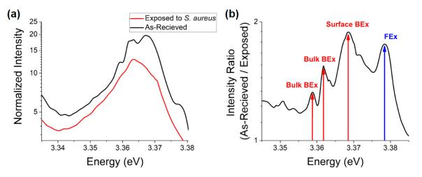
**Figure 13.** 10 K PL spectra of: (a) excitonic recombination for commercial ZnO NPs normalized to the noise floor before and after exposure to *S. aureus* bacteria in MHB growth media and (b) the ratio of the spectra shown in part (a).
