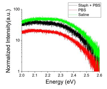
**Figure 12.** Room temperature PL spectra of deep defect luminescence regions normalized to the noise floor for a type B ZnO MP sample at 300 K after exposure to *S. aureus* in PBS as well as PBS and saline media in isolation.
