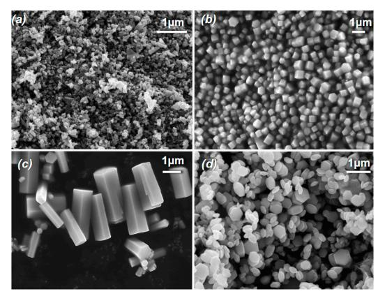
**Figure 1.** FE-SEM images of different sample morphologies: (**a**) commercial ZnO NPs; (**b**) prism-like MPs with a relative balance between polar and nonpolar free surfaces; (**c**) rod-like MPs with more nonpolar surfaces exposed; (**d**) plate-like MPs with more polar surfaces exposed.
