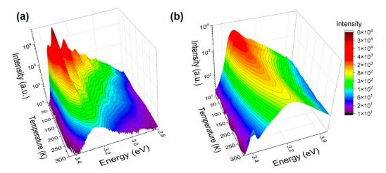
**Figure 2.** Temperature dependencies of PL spectra for: (**a**) as-received commercial ZnO NPs and (**b**) as-grown ZnO MPs.
