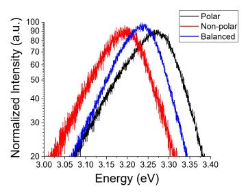
**Figure 3.** Room temperature PL spectra, normalized to the peak NBE emission, of the NBE region for as-grown ZnO MPs with different morphologies.
