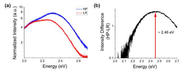
**Figure 4.** (**a**) PL spectra of deep defect emission normalized to the noise floor for as-grown ZnO MPs of differing morphology at 300 K; (**b**) intensity difference of deep defect emission for spectra shown in part (**a**).
