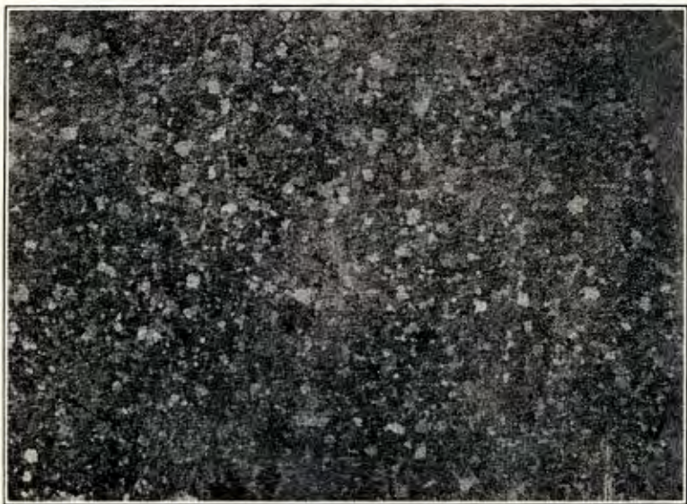
2. THE ALPINE, TEXAS, ATAXITE. POLISHED SURFACE MAGNIFIED ABOUT 4 DIAMETERS.
