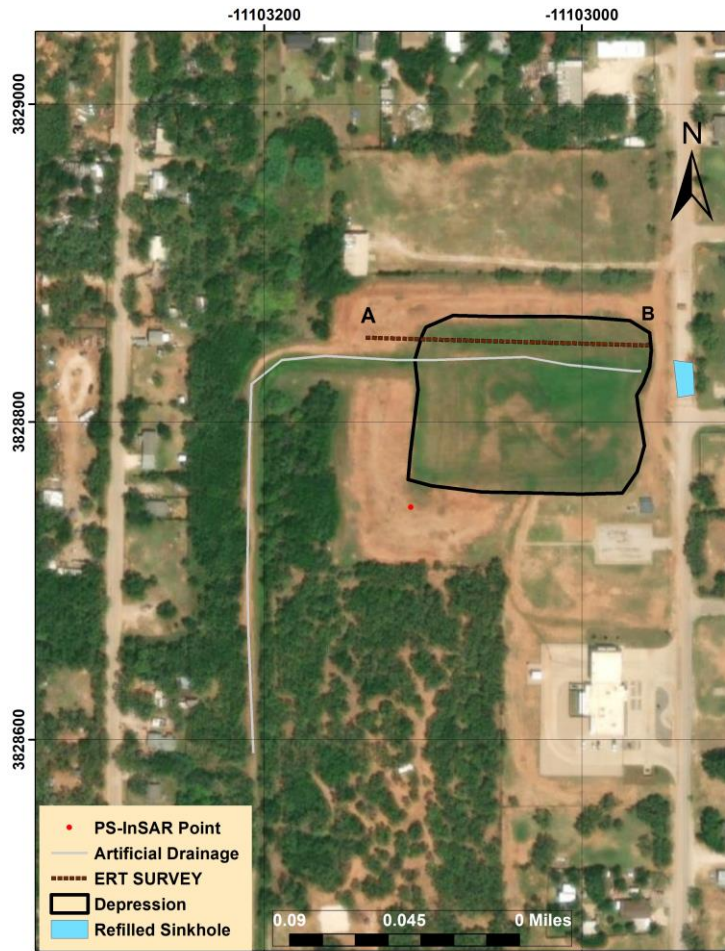
Figure 21: ERT survey (A–B) area near a refilled sinkhole site. The depression was extracted using LiDAR data (marked as black polygon), and the nearby PS point (marked as red point) revealed a displacement rate of -3.5 mm/yr.
