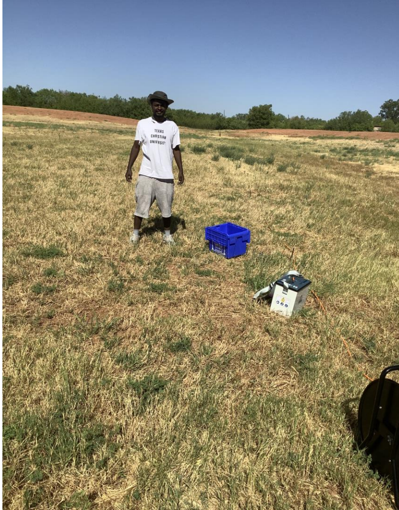
Figure 20: Geophysical (ERT) survey using the Wenner array.
