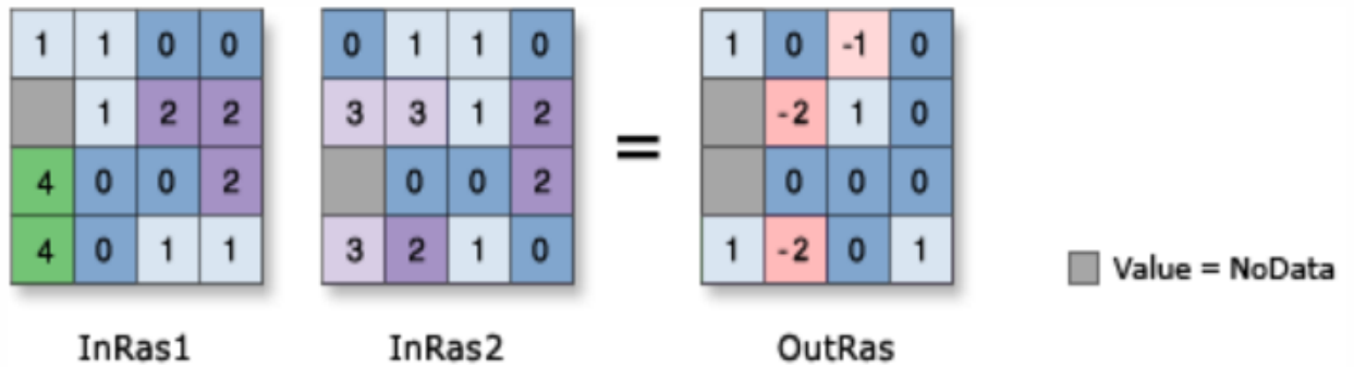
Figure 17: Illustration of the process of subtracting DEMs to delineate depressions (ESRI)
