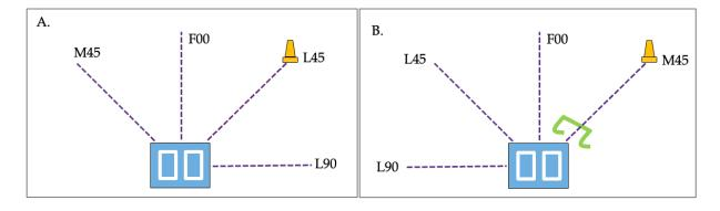
*Note.* Experimental set up for the right leg stepping to the lateral 45 direction in the absence of obstacle (A). Bottom figure (B) demonstrates the set up for the left leg stepping to the medial 45 direction in the presence of obstacle. Feet position was marked by tapes on the force plate. The walking direction for the trial is indicated by the orange cone. F00: forward, L90: lateral, M45: 45° toward medial direction, L45: 45° toward lateral direction.
