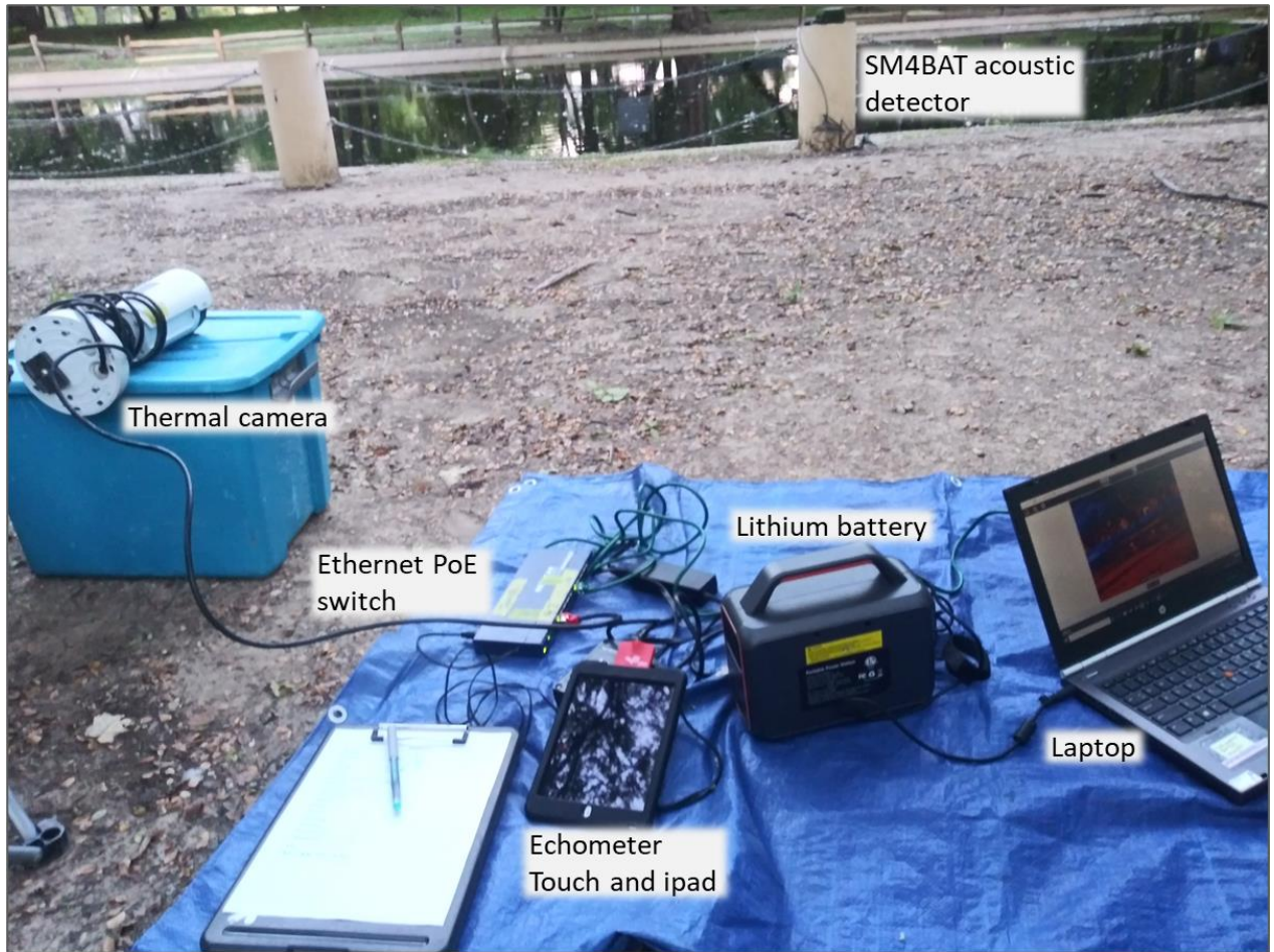
Figure 10: Thermal and acoustic equipment set up.
