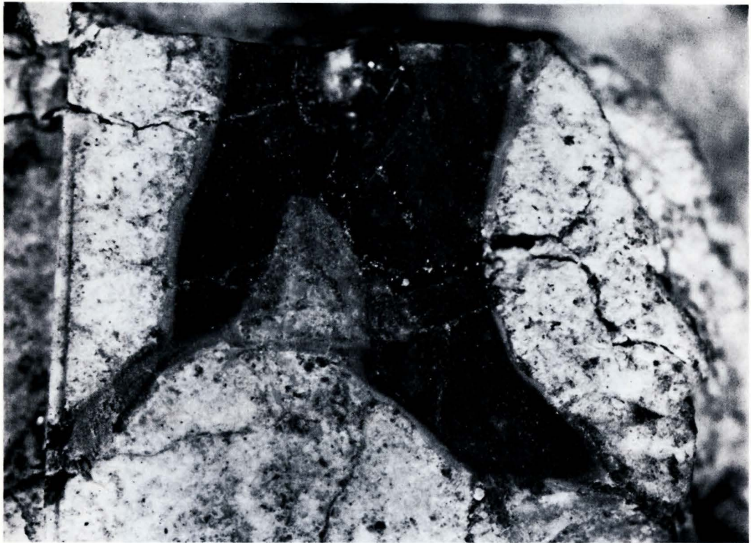
Fig. 1. Cut section of black glass in the Cachari eucrite. The glass has the same composition as the bulk of the meteorite, see Table 1. Note the bubble in the center of the glass mass. The width of the glass is 6 mm.
