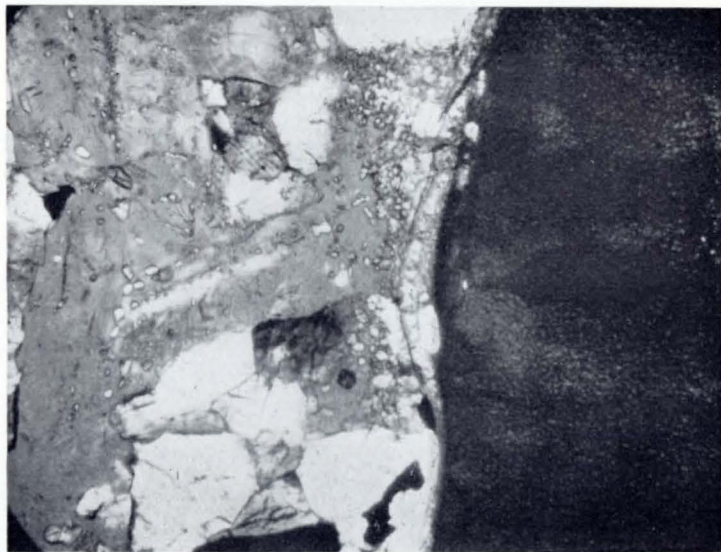
Fig. 4. Photomicrograph of contact to shock glass. The plagioclase in the center is isotropic, maskelynite, grading into normal twinned plagioclase, An 88 . The pyroxene is granulated to the left of the interface. In the adjacent glass, right, pyroxene is present as "clouds" of crystallites oriented perpendicular to the interface. Magnification 200 ×.
