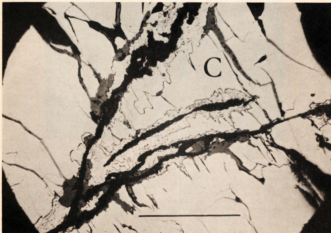
Fig. 4. Lightly shocked Canyon Diablo specimen (no. 1), showing graphitization of cohenite in cracks. The cohenite (C) has broken down to graphite (black veinlets) and kamacite (light phase surrounding the graphite, corroded to grayish oxide in places). This graphitization may be the result of conductive heating by hot ejecta. Scale bar, 100 \mu .
