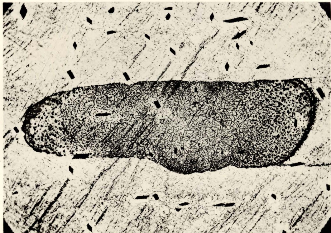
AREA OF PHOSPHORUS ENRICHMENT IN KAMACITE Sodium picrate 7 minutes and picral 10 seconds, x 100.
