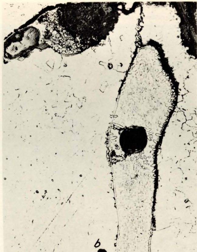
2. SCHREIBERSITE INCLUSION Picral, x 250. The round black spot is a glassy bleb.
