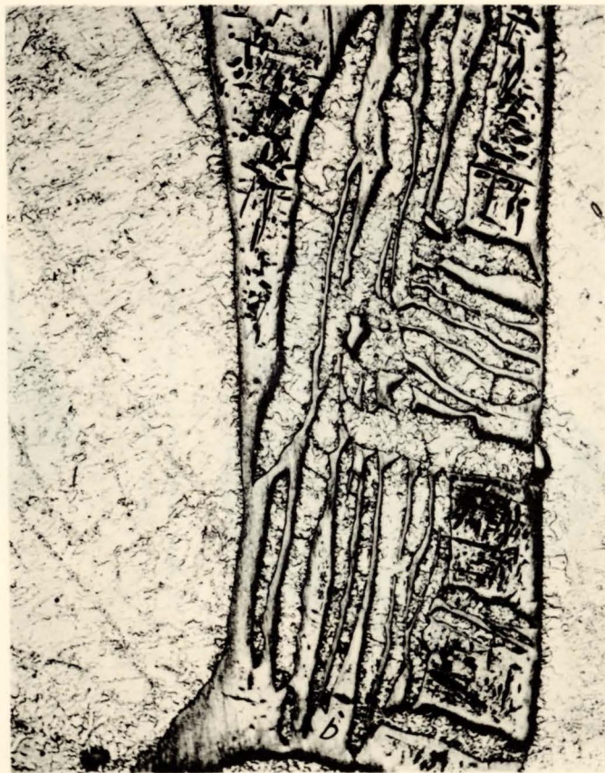
2. COARSE SKELETAL GROWTH OF TAENITE, ENCLAVING EUTECTOID PHOSPHIDE AREAS Picral, x 100.
