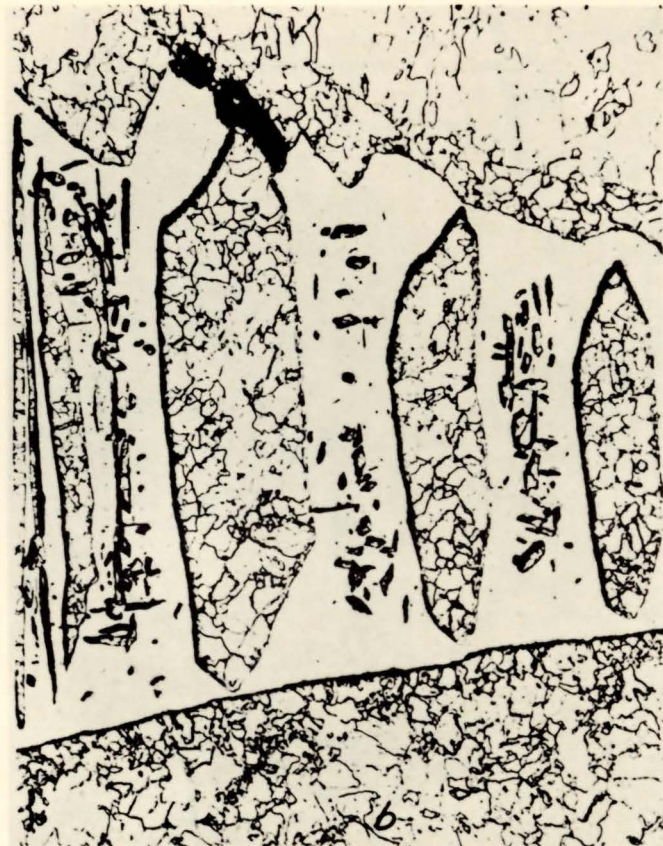
2. SKELETAL GROWTH OF TAENITE ENCLOSING EUTECTOID PHOSPHIDE. PORTION OF A LARGER AREA Picral and 10 minutes sodium picrate, x 250.
