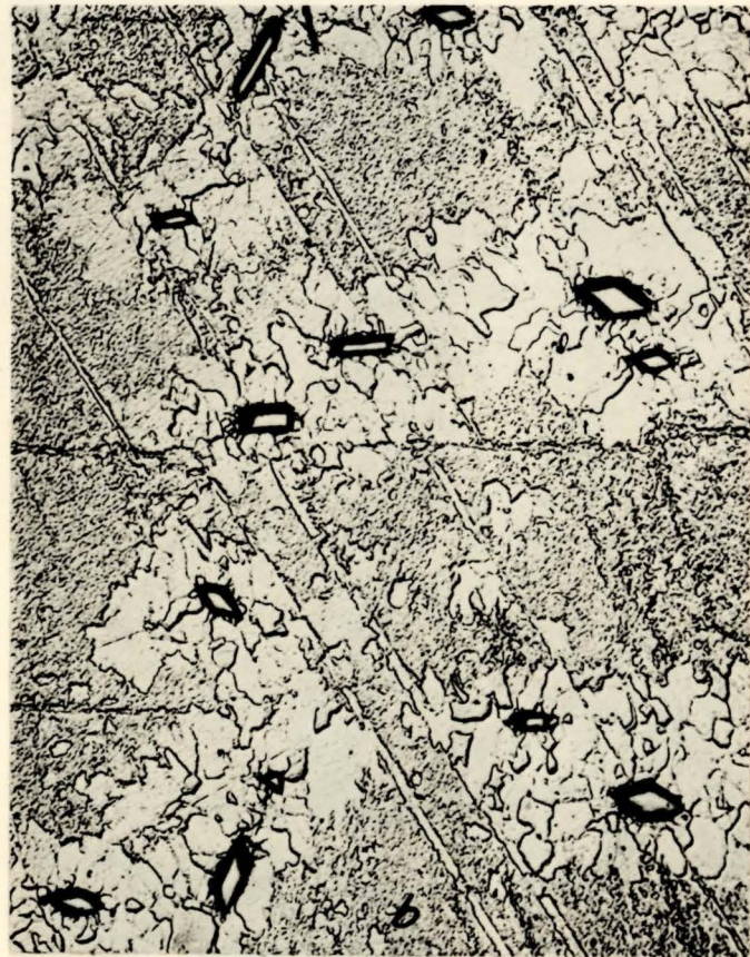
2. INCIPIENT GRANULATION AROUND RHABDITES Picral, x 200.
