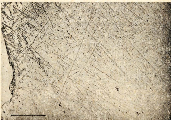
Fig. 4. Microstructure of the moderately shocked Canyon Diablo No. 3 showing \epsilon iron beginning to recrystallize, particularly on the left at the interface between the cohenite grain and the iron
