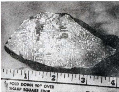
Etched meteorite from Barringer Crater showing evidences of having been heated to a high temperature.
