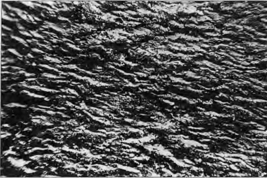
Fig. 4a. Striated relief on the lateral surface of the bomb (20X).
