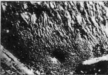
Fig. 4b. A region of surface protected from ablation by a positive surface form (20X).
