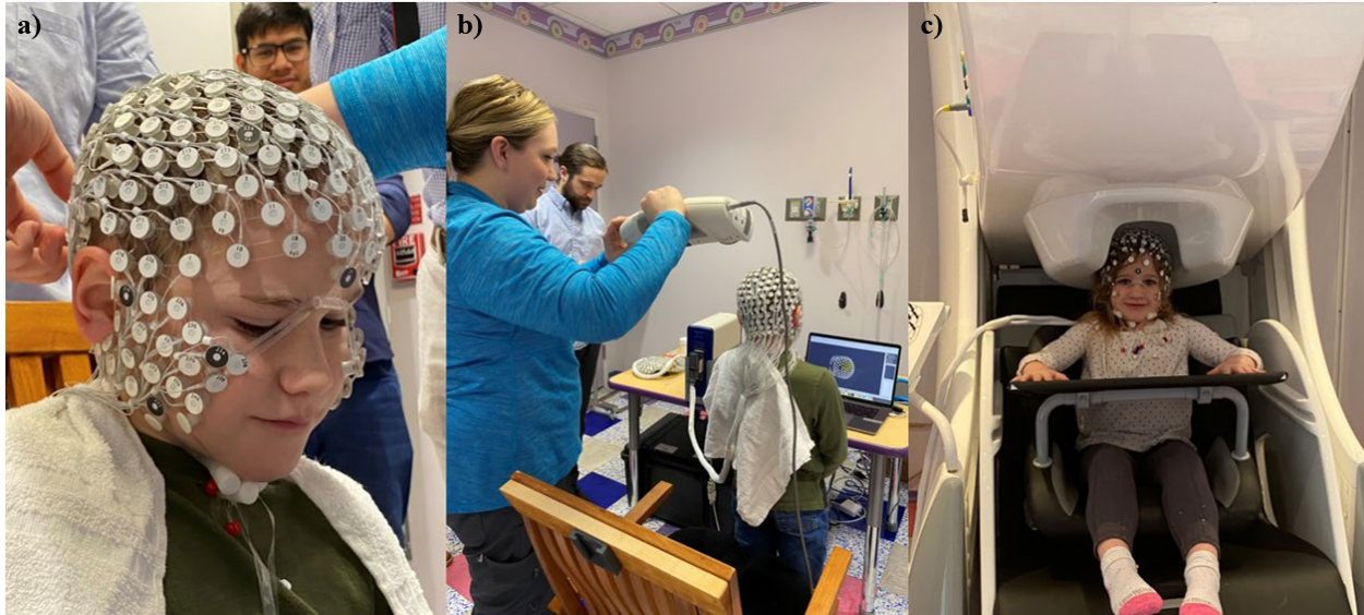
Figure 5: MEG and HD-EEG set up. (a) The Philips EGI 400 (256 electrodes) is easy to put on kids because it does not require the use of a conductive gel. Instead of using gel, you soak the net with the attached sponges in water which allows the sponges to become conductive. This procedure quick and easy, especially for children with attention deficits. (b) Co-registration procedure in order to determine the relative localization of the HD-EEG sensors with respect to the child's head anatomy. (c) The child sits comfortably in the MEG with their head placed in the MEG helmet while they sit upright.
