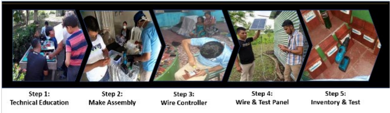
Figure 9: BTLP solar panel DEVELOPMENT & ASSEMBLY process
