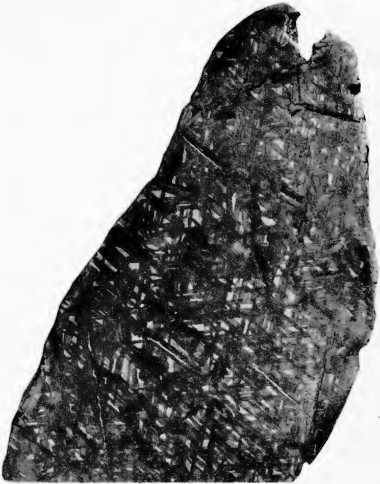
View of the Breece meteorite. Samples were taken from five of the long lathlike inclusions, Reichenbach lamellae, for X-ray, and in every case the film matched the lines on the standard schreibersite film. (Natural size.)
