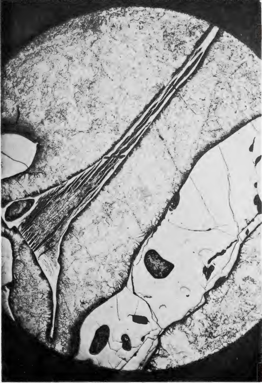
A large cohenite with the characteristic kamacite inclusions, Pittsburgh meteorite. Above this cohenite there occurs an elongated plessite area, in one corner of which is a dark island of gamma-alpha iron; in the opposite upper corner there are some delicate acicular kamacite needles. The kamacitic groundmass is granular, and small dark grains are localized along the boundary of the kamacite. (Picral, 5 percent, applied for 130 seconds; magnification, 50.)
