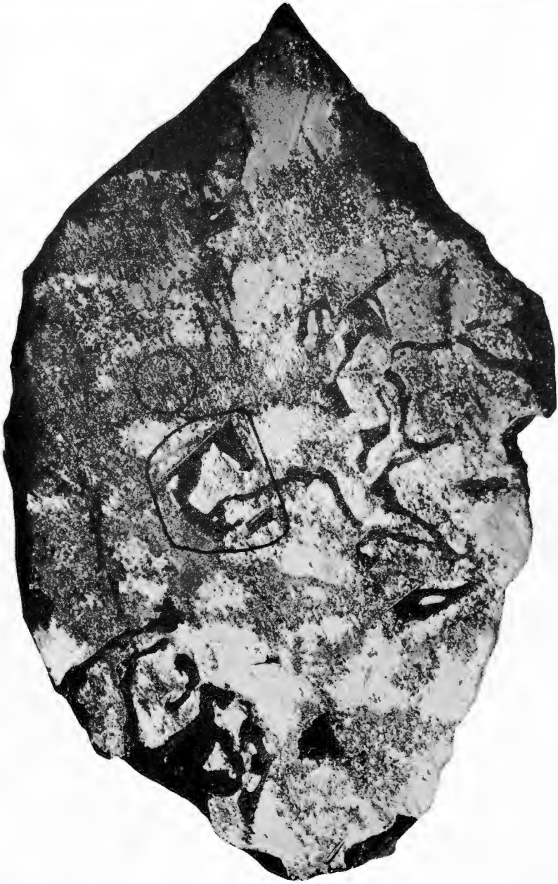
An etched cross section of the Tombigbee meteorite. Numerous irregular schreibersite bodies are dispersed in the matrix; the rhabdite inclusions are not shown. The areas selected for analysis are outlined. (Natural size.)
