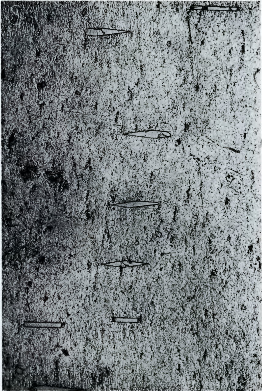
Kamacite containing rhabdite inclusions in a parallel arrangement, Pittsburgh meteorite. (Magnification, 100.)
