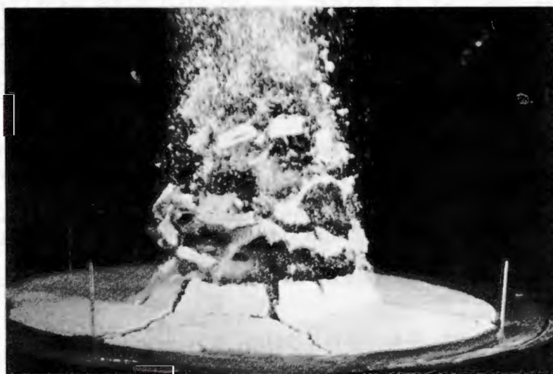
FIGURE 1. Shot 800643 showing impact (energy = 490 joules) into 1.2 cm thick layer of weakly bonded quartz particles underlain by a viscous clay slurry; note the directed ejecta plume, uptilted crustal plates, and fracture pattern (width of target is approximately 1 m).
