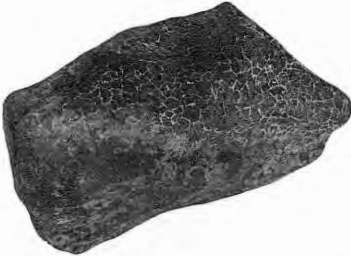
FIG. 4. Specimen three-quarters buried in wet soil, resulting in rust and exudation of molysite. Checked surface exposed. Oblique angle of light indicated by soil line. \times 1 diameters.
