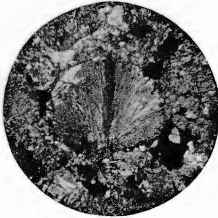
FIG. 17. Chondrule of enstatite surrounded by native iron and pyrrhotite. \times 16 diameters. Nicols crossed.
