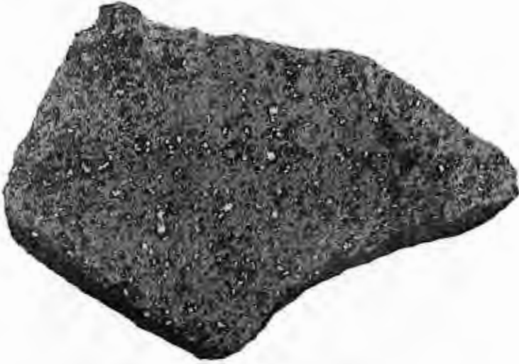
FIG. 15. Imperfect polish showing distribution of nickel-iron. At large end a chondrule encircled by minute iron grains. \times 1.7 diameters.
