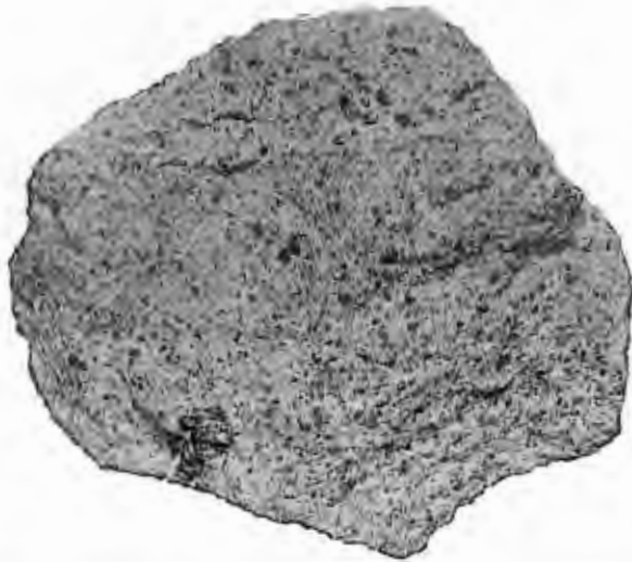
FIG. 13. Fractured surface with pyrrhotite nodule. \times 1 diameters.
