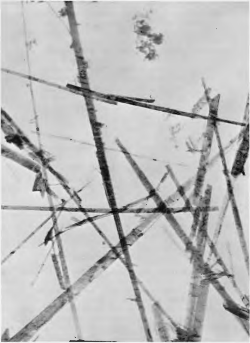
FIG. 1. Electron micrograph of material of the Erakot meteorite, showing the lath-like and tubular crystals characteristic of the chrysotile variety of serpentine. Photograph courtesy of Prof. J. D. Bernal, Birkbeck College, London. \times 24,000 .
