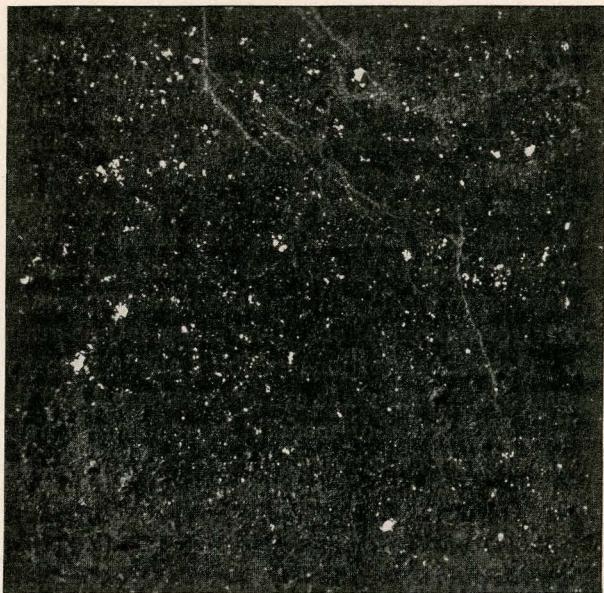
Fig. 3. Polished surface of Long Island meteorite showing size and distribution of metallic grains. Fully half of these are troilite. The light irregular lines mark the position of fractures of no significance. \times 45 .
