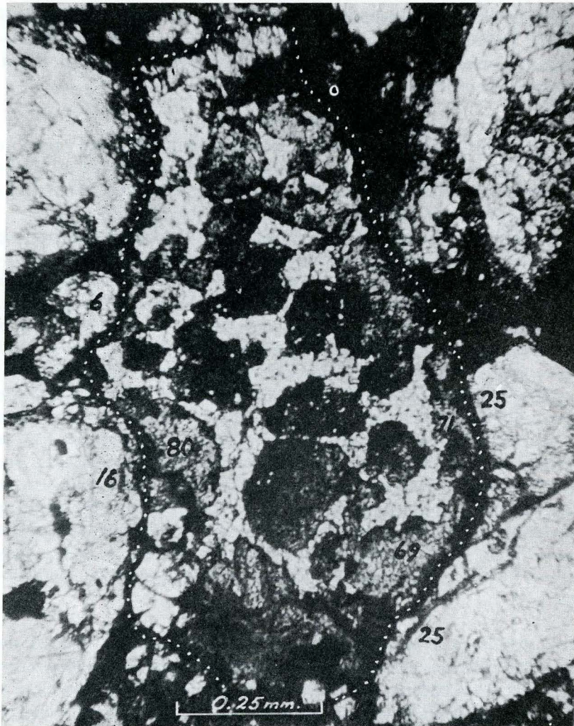
FIG. 4. Photomicrograph, in plane light, of a chondrule fragment in Mezö-Madaras, consisting of olivine (gray), clinoenstatite (white), and merrihueite (black areas). The chondrule is outlined with a dotted line. Olivine compositions (numbers) are given in mol % Fa.
