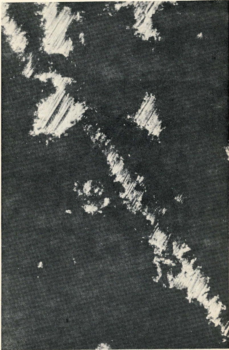
Figure 4. Photomicrograph of a portion of the veinlet shown in Figure 3. Polishing grooves are conspicuous in the Ni-Fe.
