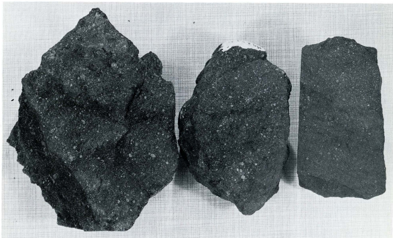
FIGURE 1.—Hand specimens (left to right) of Murchison, Murray, and Mighei C2 meteorites. Murchison and Murray show a closely similar content of inclusions, in contrast to other C2s such as Mighei. The Mighei specimen is 7 cm long.
